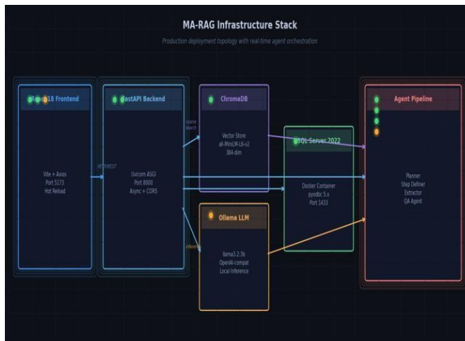
Figure 5. MA-RAG infrastructure deployment topology — FastAPI backend orchestrating ChromaDB, Ollama LLM, SQL Server, and the four-agent pipeline.
